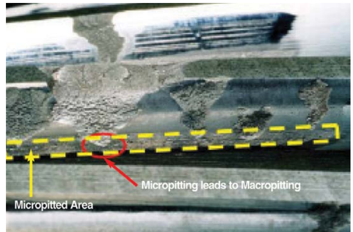
Figure B: Micropitting leading to macropitting
