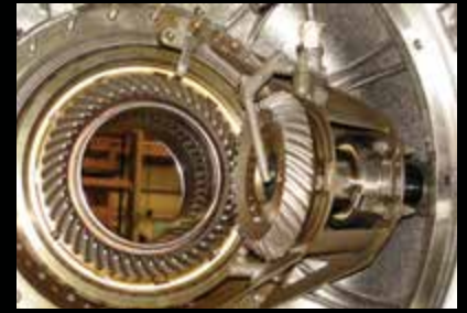
Rear part of forward sump. Sump walls and the inlet gearbox, in situ in the fan frame, were exceptionally clean.
