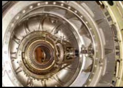
Rear part of forward sump. Sump walls and the inlet gearbox, in situ in the fan frame, were exceptionally clean.
