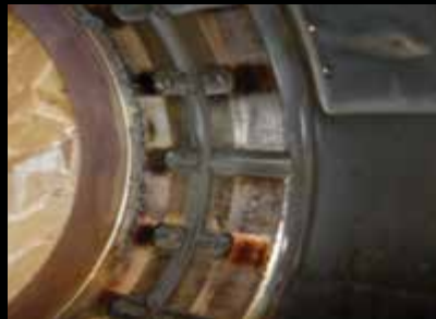
Bearing #4. Oil supply grooves under the inner race were free of sludge and deposits. A few small particles were trapped by centrifugal forces in the forward circular groove. The small feeding holes were free of clogging.
