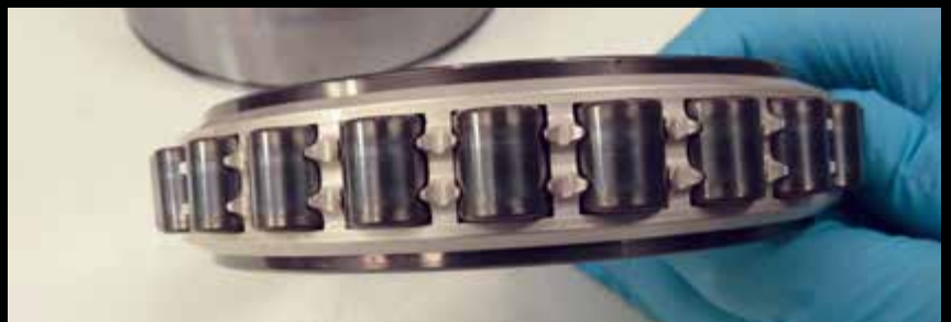
Bearing #5. Laboratory inspection found bearing #5 without defect and serviceable.
