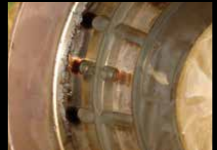
Bearing #4. Oil supply grooves under the inner race were free of sludge and deposits. A few small particles were trapped by centrifugal forces in the forward circular groove. The small feeding holes were free of clogging.
