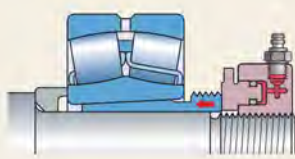
HMV ..E nut screwed onto the shaft for driving in a withdrawal sleeve.
