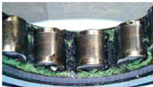
Lubricant degradation caused by electrical discharge currents
