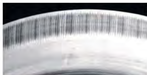
Fluting marks characteristic of electrical erosion in bearings
