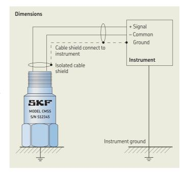
Fig. 2. Grounding at instrument side.
