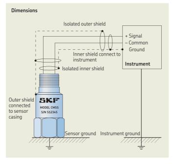
Fig. 4. Grounding with double-shielded cable.
