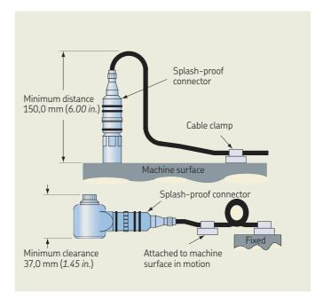
Fig. 5. Cable anchoring.
