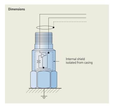
Fig. 1. Electronic circuit isolated from sensor casing.
