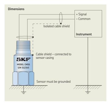
Fig. 3. Grounding at sensor side.
