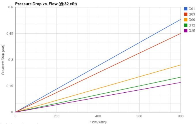
Fig. 1: Flow vs. Pressure drop
